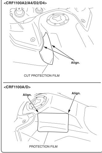
Install the right side of the protection film in the same manner as the left side. 7. Remove the straps as shown.
